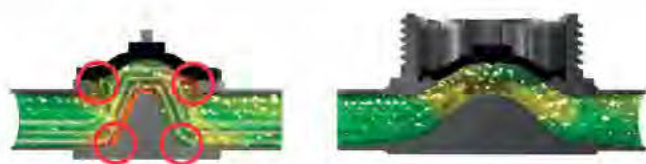
Figure 3. The new generation diaphragm valve (right) has minimized sharp corners compared to the traditional valve (left) which has sharper corners (circled). The smoother corners reduce turbulence and thereby pressure drop.
