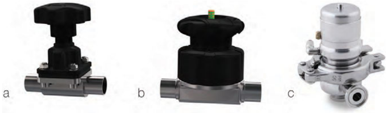
Figure 1. Comparing the four bolts of the traditional diaphragm valve (a) to the centralized thread on the new generation diaphragm (b) and the radial diaphragm with clamp assembly (c). The centralized thread provides quick, easy and safe installation as well as service of the valve.
