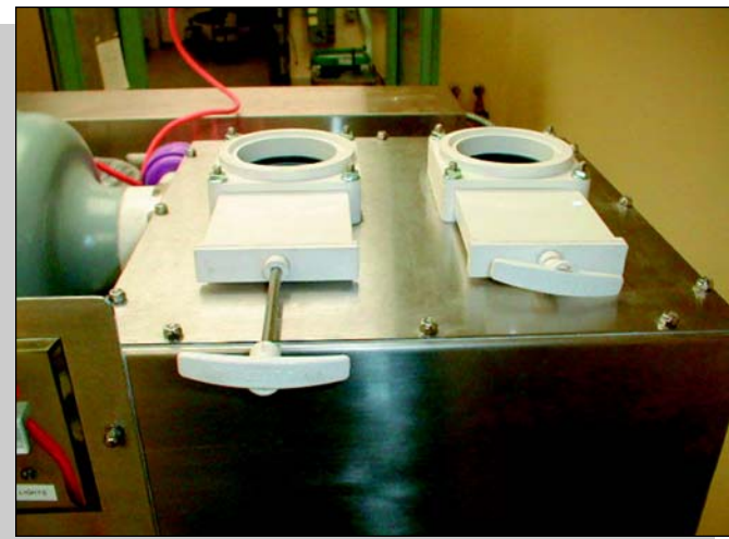
Figure 6. Tablet press isolator slide gates for controlling isolator air pressure differential.
