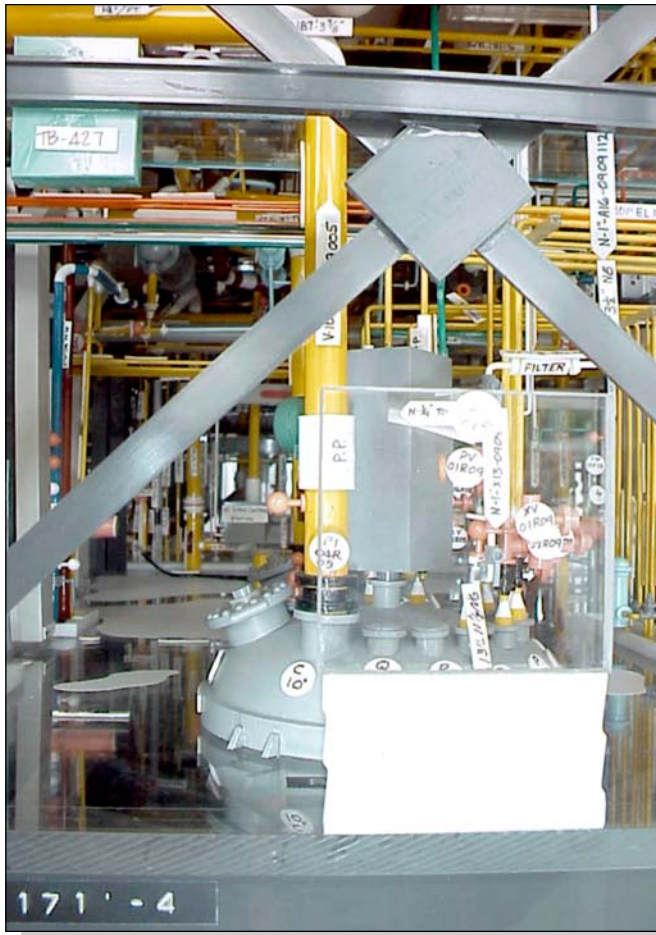
Figure 1. Top of a reaction vessel - digital photograph of a plastic model.
