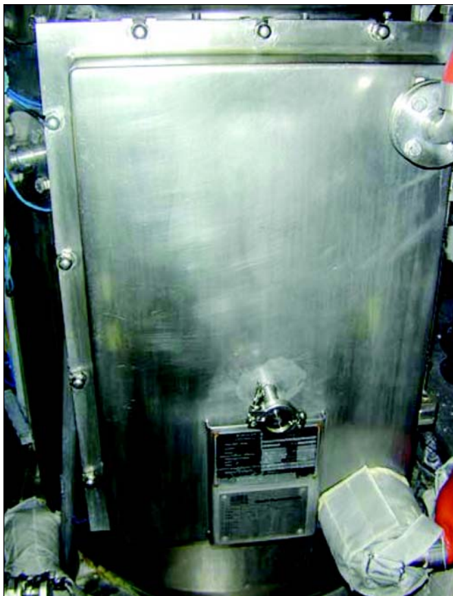
Figure 6. Nütsche dust filter showing the access cover fitted with a cleaning nozzle.
