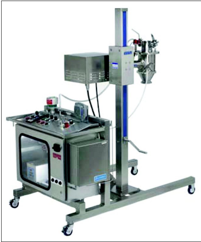
Figure 2. Mobile inert mill system with oxygen monitoring controls.
